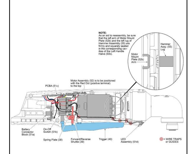
AS AN AID TO REASSEMBLY, TAKE NOTICE OF WIRE ROUTING AND POSITION IN WIRE GUIDES AND TRAPS WHILE DISMANTLING TOOL.
